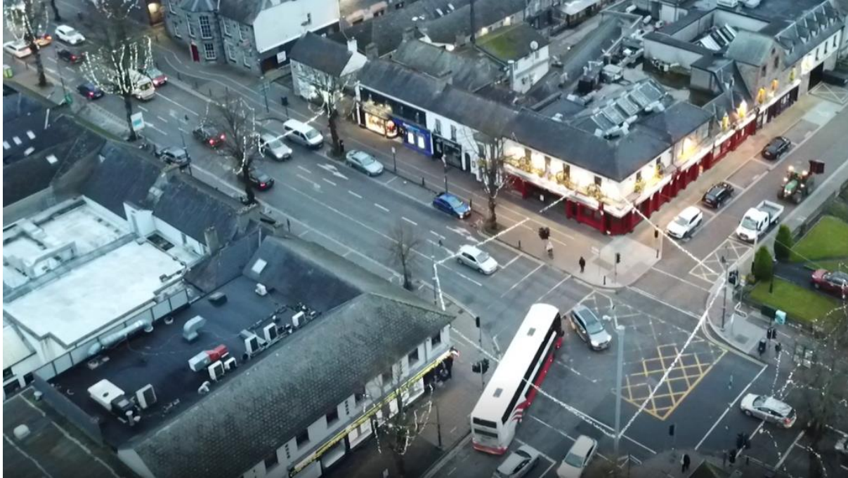
Figure 4-4: Turning difficulties for buses travelling from Mill St to Main St
